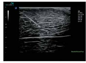
Needle Vision™ Plus providing better visualization of a needle tip and shaft with Beam Steering technology
