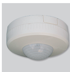
CPFL-S / CPFL-E Presence detector for ceiling mount, sensitive to infrared radiation by bodies in movement, with a 360° detecting angle. Power supply: 1-230 V.
