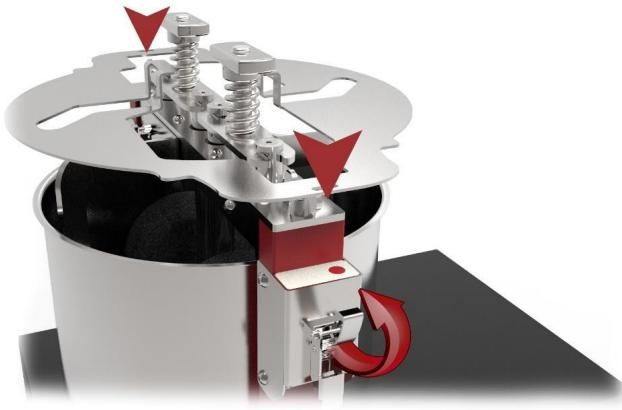
7.5. Do not start melangeur when the stones are dry (!). This may cause rapid deterioration. During the grinding, axes of the millstone must be covered with the mass — this determines the minimum loading capacity of melangeur (!).
