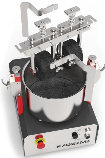
7.3. Before starting the rotation, you need to turn on the circuit breaker located on the rear wall of the body (under the casing). Also check button (4): if it turned on — rotate it clockwise to turn off.
