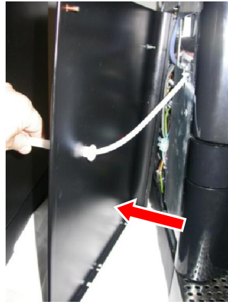
Insert the inlet milk pipe into the pass bulkhead, and then trough the side panel hole.
