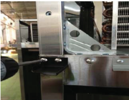
C-1. Disassemble the top hinge (left).
