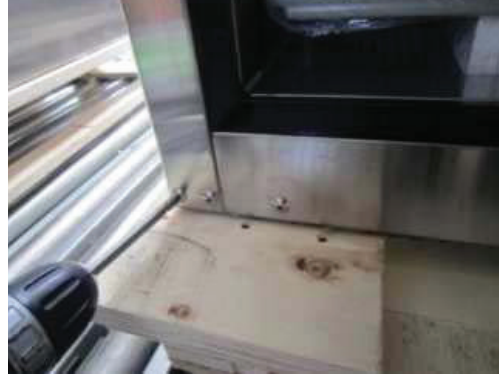
C-2. Disassemble bottom hinge (left).
