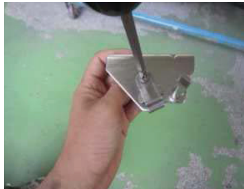
C-2. Disassemble bottom hinge (left).
