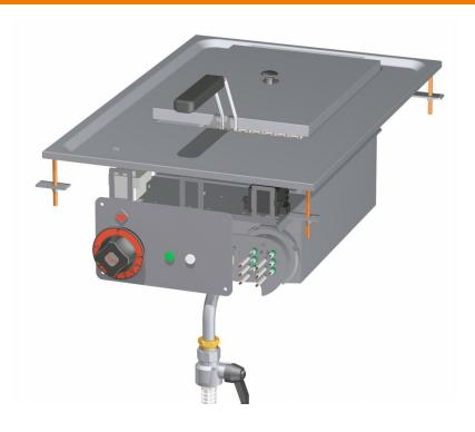
Construction - Fabricated using CrNi 18/10 AISI 304 grade Stainless Steel Scotch-Brite Satin polish Finish, incorporating 2 mm thick worktop, chromed details. Model - Professional Electric Fryer. With single or Double tank to include both basket and lids, tank filter with basket support. Double Thermostat for operating and over heat safety. Maintenance - Easy tank cleaning by rotating heating element. Fittings -Fixing system.
