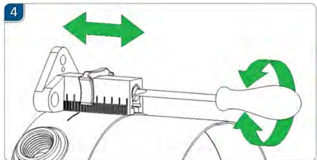
**For plasterboard application remove the clips and turn the supports backwards**
