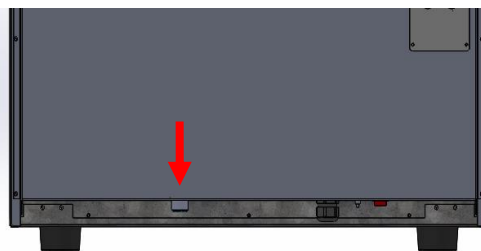
Figure 4. Water intake for Bakershop 4,6,10 (600x400)
