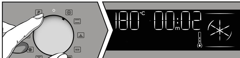
The temperature rise starts immediately. The time indicator tells you how long the oven has been running. The oven heats up and the temperature indicator flashes. A series of beeps will sound when the oven reaches the programmed temperature.
