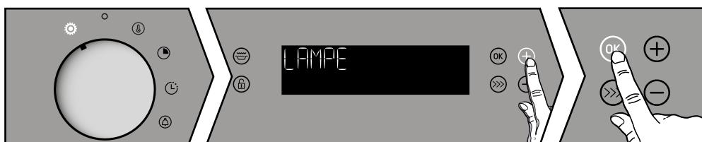
Press the **OK** key to confirm your choice. Using the + and - keys activate or deactivate the various parameters, see table.
