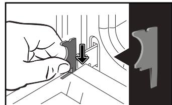
Use a tool (screwdriver) to press the slots A in order to unclip the glass panel. Remove the glass panel.
