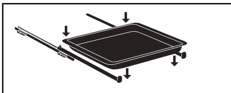
To remove the rails, remove the shelf runners again. Slightly prise apart the bottom of the tabs fixed on each rail to release
