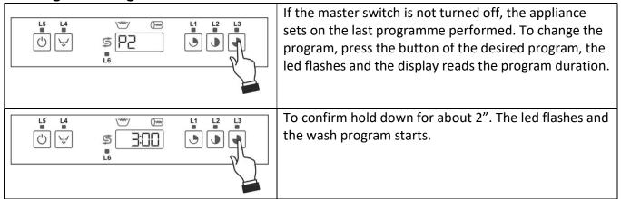
If a programme is already running, it can be changed by first switching the appliance to pause status (by pressing one of the buttons for 2") and then selecting the programme required.
