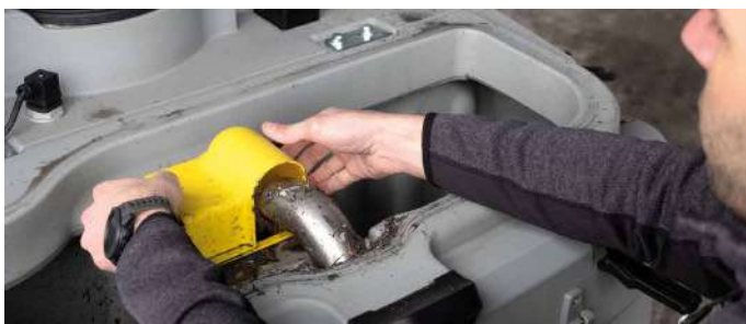
Basket filter to catch any debris, preventing it from settling on the bottom of the recovery tank.
