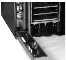
Electrical parts integrated in the front left column under the control panel to avoid the waste of space occupied by the "traditional" external electric boxes
