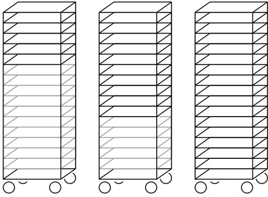
B-FS electric version is the first three-section rotary rack oven (patented) which allows to reduce the consumptions by 33% or 66% when baking of a complete rack is not needed: you can decide whether to bake 5, 10 or 15/18 trays and thus to use 1/3, 2/3 or 3/3 of the power. No more money wasted on the unnecessary consumption of your old oven!
