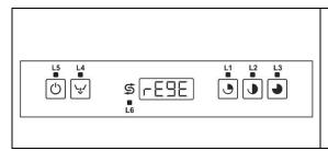
If "rE9E" appears on the display, it indicates that the machine is carrying out a resin regeneration cycle, which lasts approximately 90 seconds. It is normal for the machine to fill or drain water automatically during this procedure, even if it is not carrying out a washing cycle.
