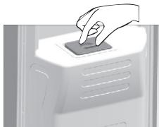
➲ When taking water from a new refrigerator for the first time, press and hold the ice discharge button, take the first 1 ~2 L of water and discard, and then take water for drinking;
