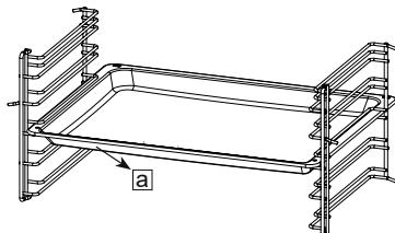
Accessories should be placed between two racks and the side with a inclination should face the door of the appliance.
