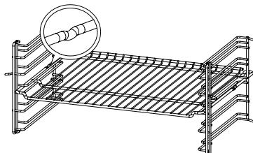
The cavities on the wire rack prevent it from falling off the racks and ensure the safety.
