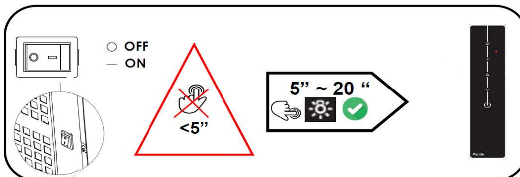
If it takes more than 20 seconds to synchronize the control, the hood switchboard closes the reception and does not record any code, you must repeat the process, making sure to press the key between 5 "and 20".
