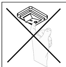
DO NOT ACTIVATE THE SWITCH ON, UNTIL YOU REACH STEP **(12)** OF THE INSTALLATION PROCESS.
