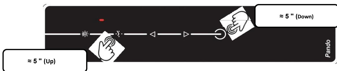
3. In maintenance mode, while the hood body module containing the panels and filters moves up and down, acoustic and visual signals are emitted, **the acoustic is a continuous 2-second beep with intervals of 1 second**, the visual is the led control pilot light for the motor, which will flash red.
