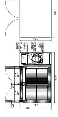
heat discharge.) B: The cooling effect depends on space to meet the air flow and water supply pipe,drain pipe,and reserve additional space 10cm at place the equipment connect the installation requirements.(Air instructions, properly install and A: Please follow the the installation site to meet the
