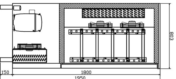
A: Please follow the instructions, properly install and place the equipment, connect the water supply pipe, drain pipe, and reserve additional space 10cm at the installation site to meet the installation requirements. (Air cooling equipment needs more space to meet the air flow and heat discharge.)
