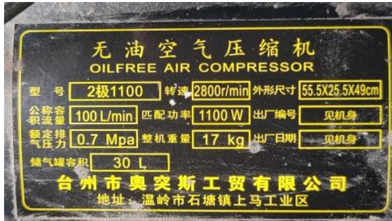
PIC 2 Air Compressor Nameplate
